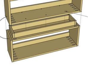
Drill holes in upper shelf of middle assembly. See the illustration in Step #1 for hole locations.
